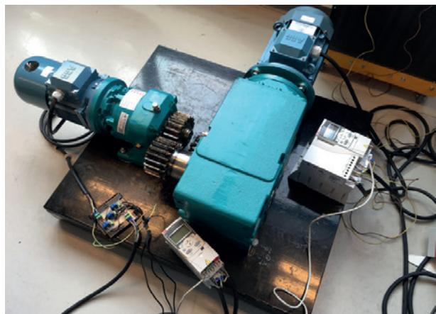
Figure 1: Laboratory setup with pitch drive (left) and load motor with bph gearbox (right)
