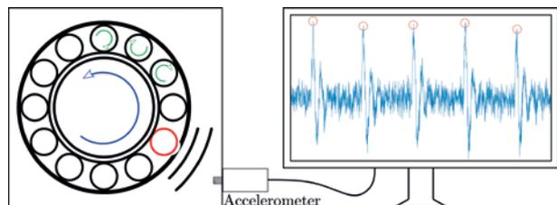
Figure 1: The bearing vibration is monitored using an accelerometer attached to the bearing housing.
