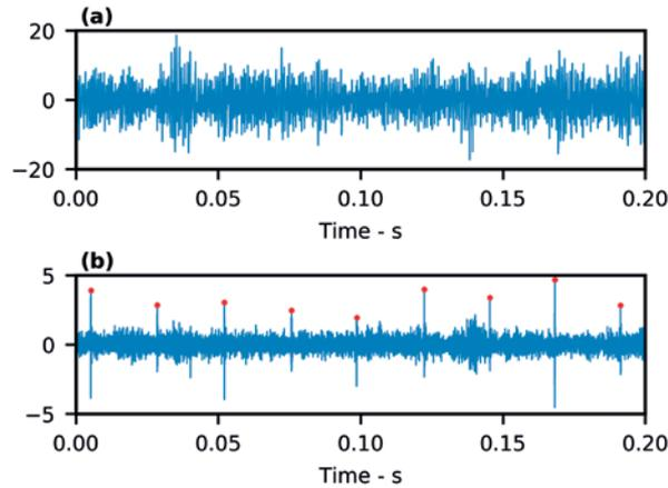
Figure 2: The raw vibration signal is filtered using an autoregressive model to highlight bearing faults. (a) The raw signal. (b) The filtered signal with red dots signaling the bearing impact vibration.
