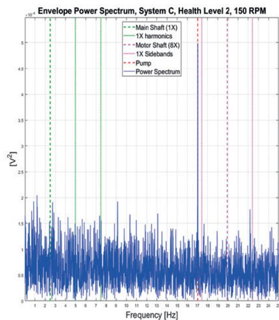
*Left: Acceleration envelope power spectrum. Clear peaks at motor and main shaft speeds with harmonics and sidebands. Right: AE envelope power spectrum. Clear peak at lubrication pump frequency, not visible in the acceleration spectrum*
