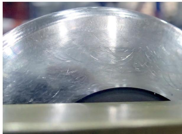
*Arc-shaped scratches observed on the roller end of a worn axial tapered roller bearing from a top drive.*
