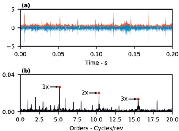
Figure 3: The envelope spectrum is analyzed to detect faults in the bearing. (a) Filtered vibration signal with the corresponding envelope. (b) The envelope frequency spectrum indicating an outer-race fault.
